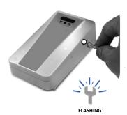
Stand to the right out of the detection beam and adjust the Half Flush cycle time by holding the Magnetic Wand against the right side Magnetic Target until the desired water release is achieved.
