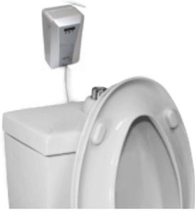
Position the Sensor on the wall behind the tank such that it is high enough to "see" above any obstacles, yet low enough to detect a person sitting on the toilet.
