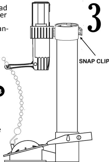
Check the relative alignment of both lever arms and chains to ensure there is no interference, adjust as necessary, then secure the motor mount snap clip.
