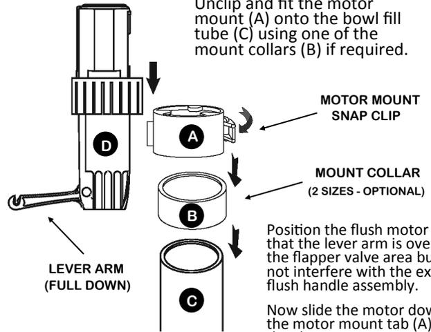
Position the flush motor (D) so that the lever arm is over top of the flapper valve area but does not interfere with the existing flush handle assembly.
