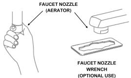
FEEL OR LOOK UP INSIDE THE FAUCET SPOUT TO ENSURE THAT ANY WASHER, O-RING GASKET OR FILTER SCREEN IS REMOVED
