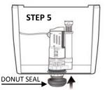
Stretch the tank-to-bowl rubber donut onto the flush base flange and nut. Note that this is a general purpose gasket. In some cases where a custom gasket is used, the old gasket will need to be reused or purchased from the manufacturer.
