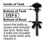
If the spacing between the tank and bowl is tight, then omit the center washer and
