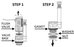
Separate the dual flush Remove the large nut valve from its base by and washer from the rotating the flush valve base, but leave the until its retaining tabs rubber gasket in place. align and it pulls free.
