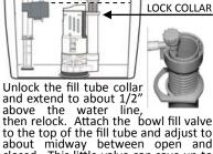
then relock. Attach the bowl fill valve to the top of the fill tube and adjust to about midway between open and on, press down on the valve and closed. This little valve can save up to an extra gallon on each flush.
